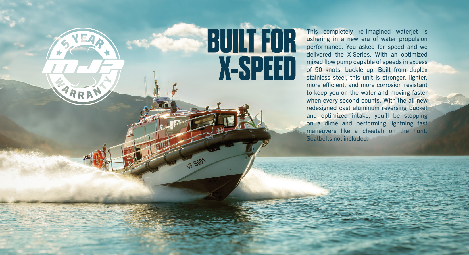
Above: STEM Marine 12M Fire/Rescue Craft featuring dual MJP 310X waterjets. Photo courtesy of STEM Marine.
